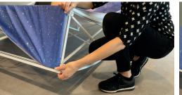
9. Start in the 4 corners of the frame, to divide the tension.
