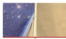
8. Attach the fabric by pushing the silicone edges in the grooves.
